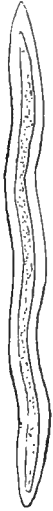
FIG. 116. — A wood fiber, consisting of a much elongated cell with thick woody walls.
